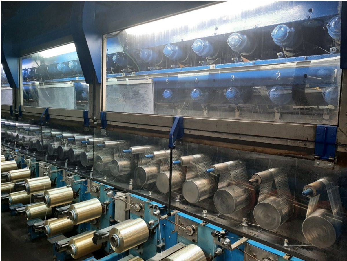
Fig. 9 Modification of drying space cover on spinning machine at dry side
