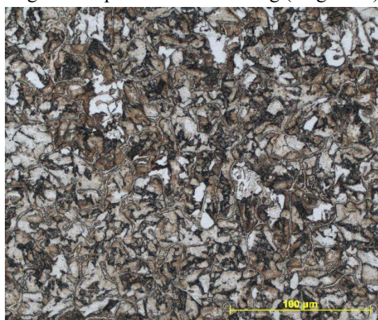
Fig. 18 Microstructure of sample E3, magnification 500x, ferrite, pearlite
