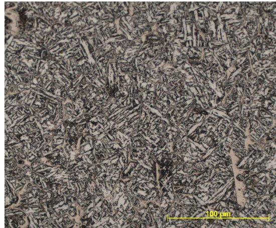
Fig. 14 Microstructure of sample E2, ferrite, bainite, (mag. 500x),
